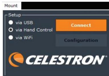
Wait for the Align Mount window to pop up after you have selected Connect. Check and make sure the Status box in the bottom right corner in the Mount section displays in green font that you are connected to CPWI.
