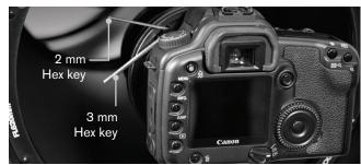
7. If the star pattern is thin on one side, adjust the collimation screws so that the star moves towards the thin side, then adjust the position of the astrograph to re-center the star. Repeat this until the defocused star image is concentric.
