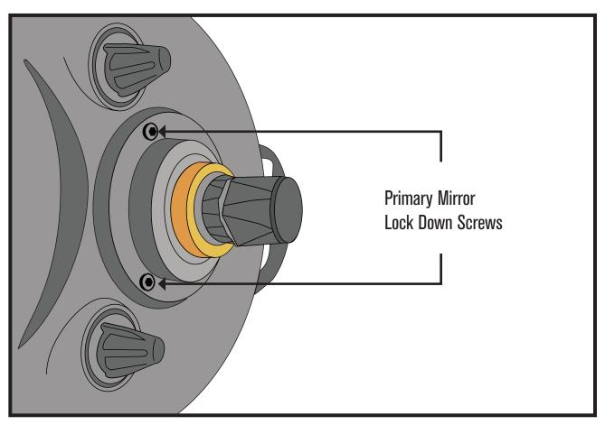
In order to facilitate secure shipping of the EdgeHD 14" tube, the primary mirror has been locked in place with two screws preventing the focus knob from turning. To release the primary mirror, use the included 3/16" Allen wrench and loosen both screws until they float freely in the rear cell casting.
